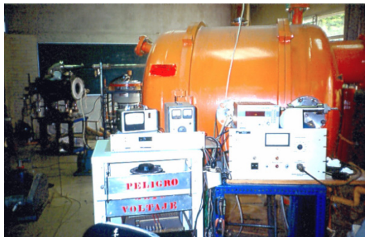
Fig. 1. Photograph of vacuum chamber, high voltage source, and vacuum gauges
