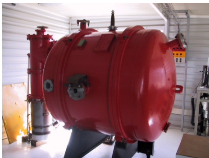
Fig. 4. Photograph of the vacuum chamber and diffusion pump for high vacuum
